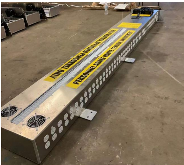
Picture above: PDU side view
